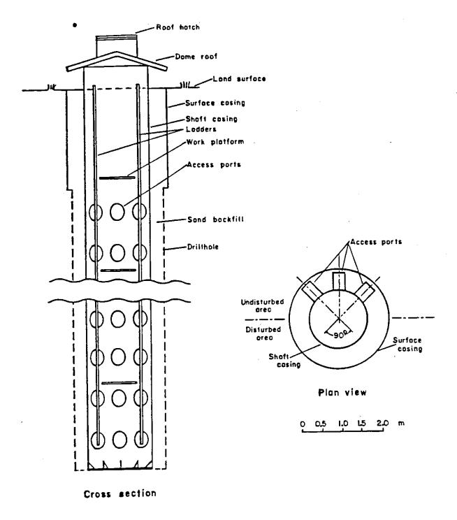
Figure 2. Cross-sectional and plan views of the vertical monitoring shaft.
