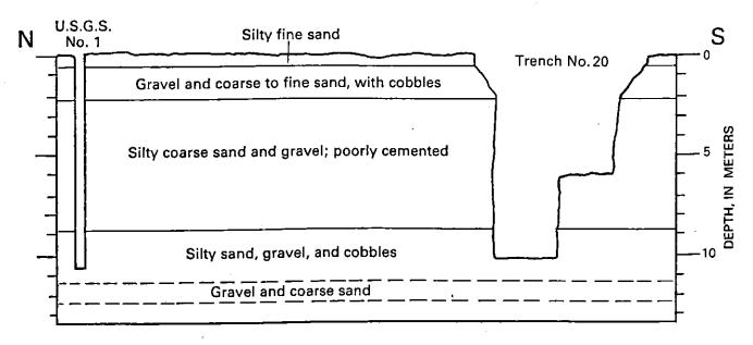
Figure 27. Diagrammatic geologic section of shallow unconsolidated deposits at waste-burial site. Vertical exaggeration=7×.
